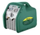
Power: 3/4HP Voltage: 220V/50HZ, 1450 Oil-free compressor, suitable for all commonly-used refrigerants. Self - purification function, can remove the residual refrigerants in the machine Low pressure protection, automatic shutdown High - pressure protection, reset button
