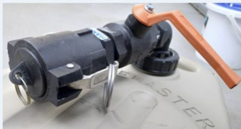
Bayonet type cap fitted to isolating valve
